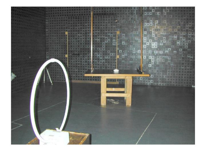
Photograph 2 Radiated emissions measurement test setup
