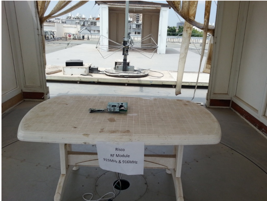
Figure 6. Radiated Emission Test
