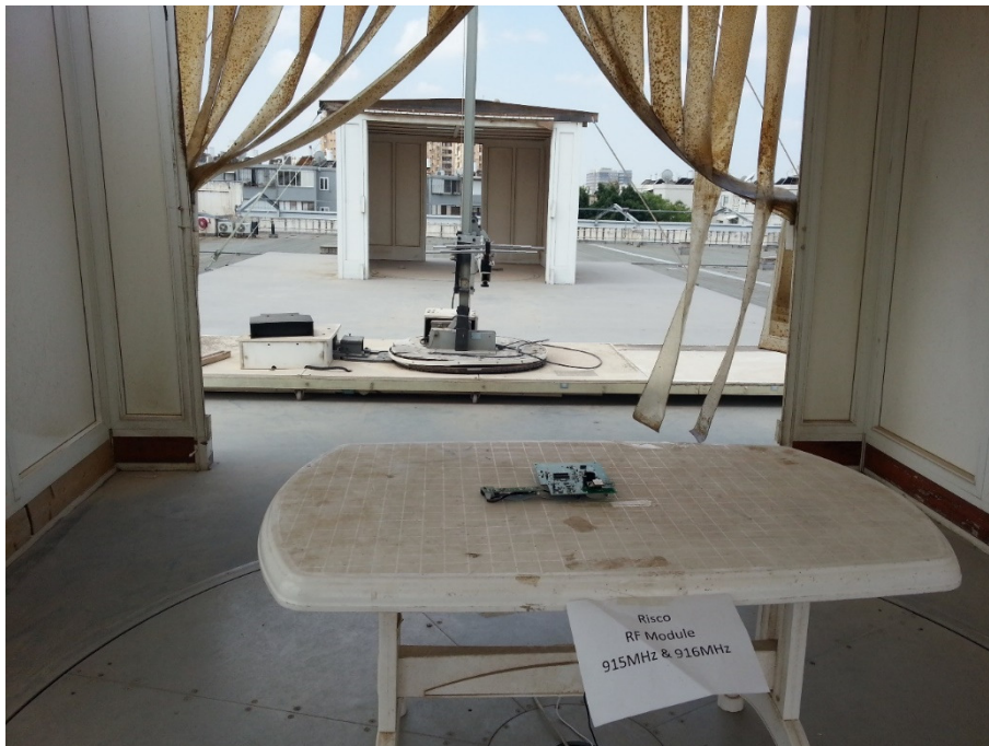
Figure 5. Radiated Emission Test
