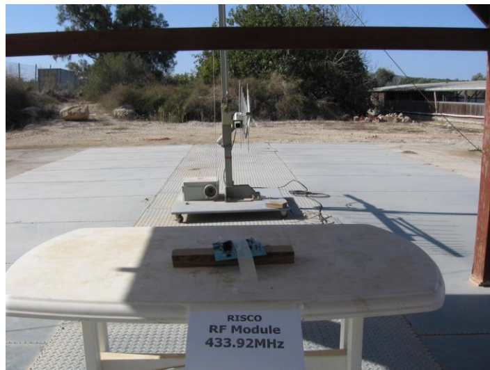
Figure 3. Radiated Emission Test
