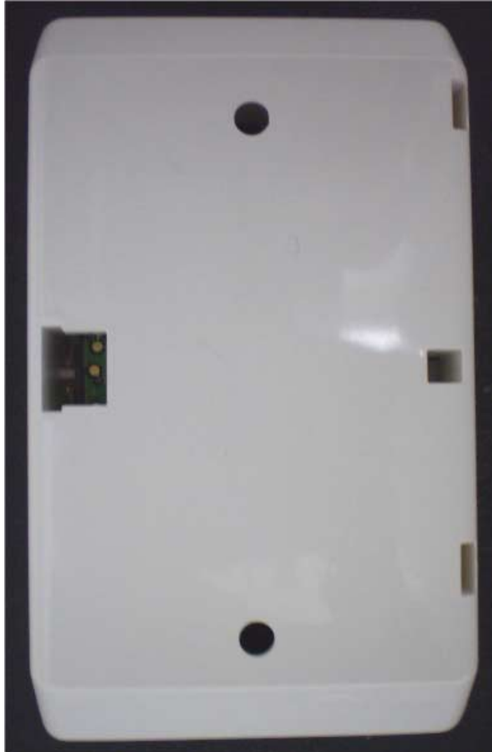
Photograph No.2 Wireless VITRON glass-break detector rear side view
