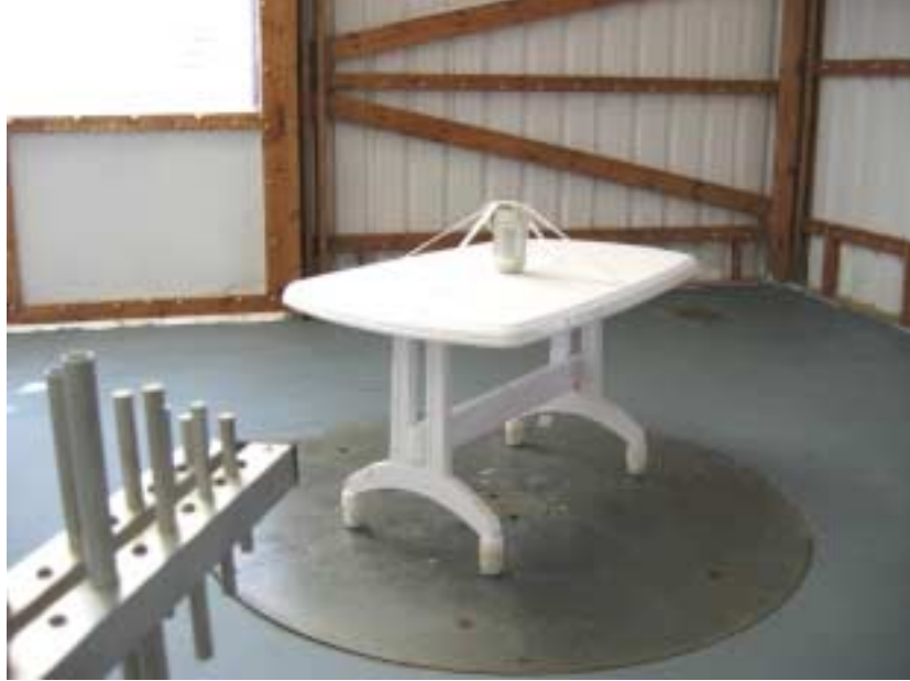
Photograph No.5 Spurious emissions field strength measurement setup at the OATS in 30 -1000 MHz
