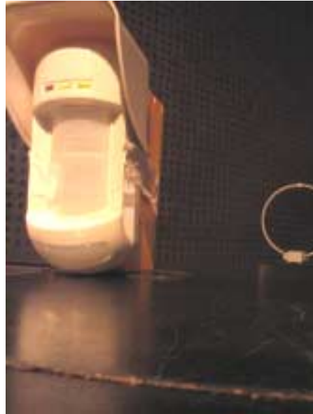
Photograph No.4 Spurious emissions field strength measurement setup in the anechoic chamber, EUT close view
