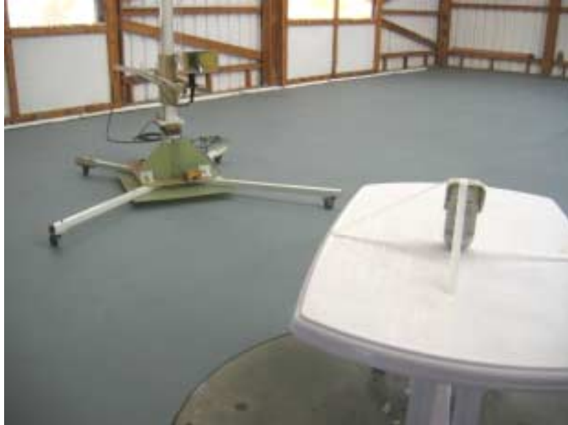
Photograph No.6 Spurious emissions field strength measurement setup at the OATS above 1 GHz
