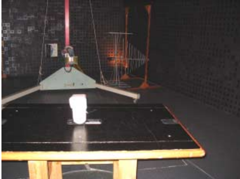
Photograph No.3 Spurious emissions field strength measurement setup in the anechoic chamber above 1 GHz
