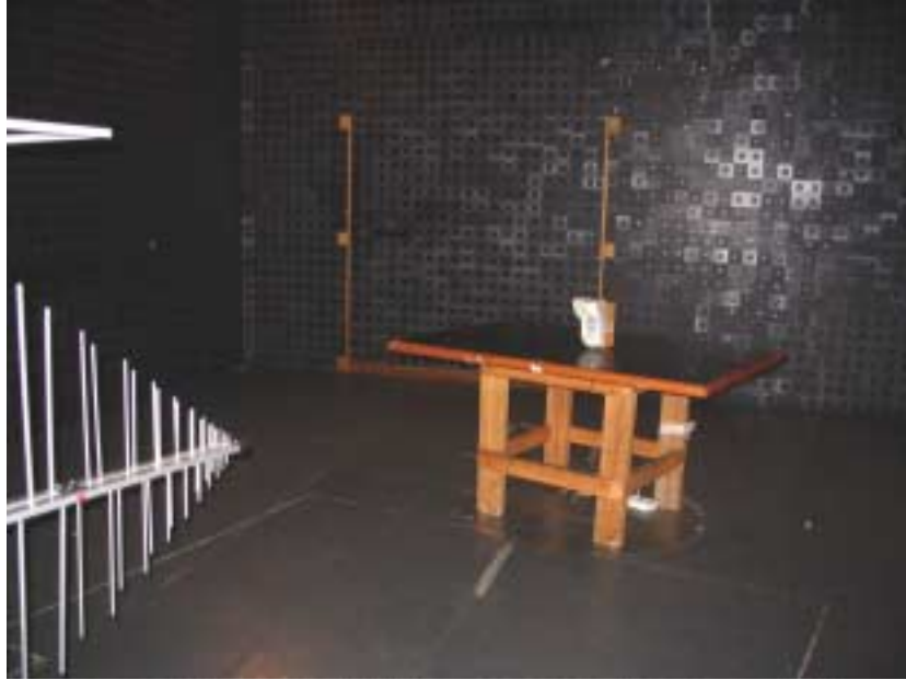
Photograph No.2 Radiated emission measurement test setup in the anechoic chamber in 30 -1000 MHz
