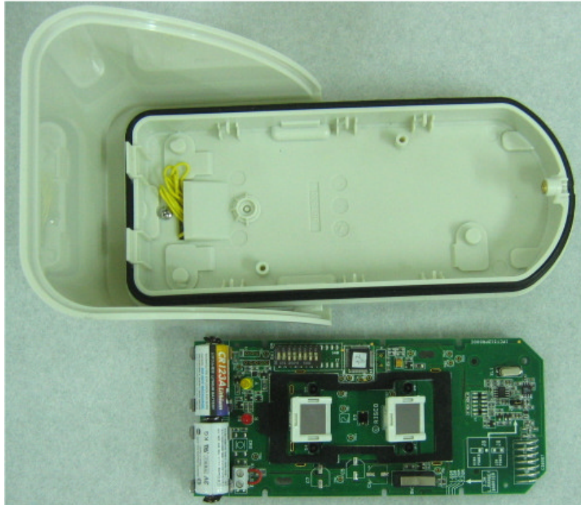
Photograph No.3 Main PCB removed from back cover view
