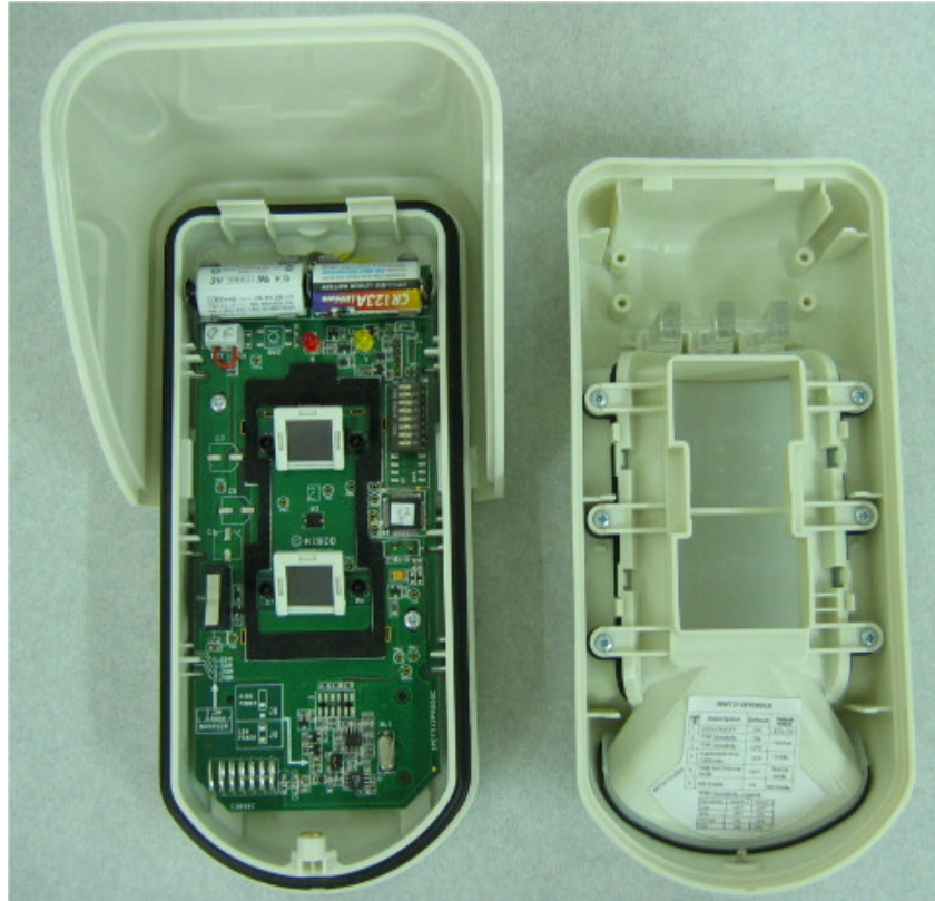
Photograph No.1 Wireless WatchOUT PIR detector internal view with front cover removed
