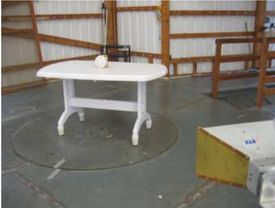
Photograph No.3 Spurious emissions field strength measurement setup above 1 GHz
