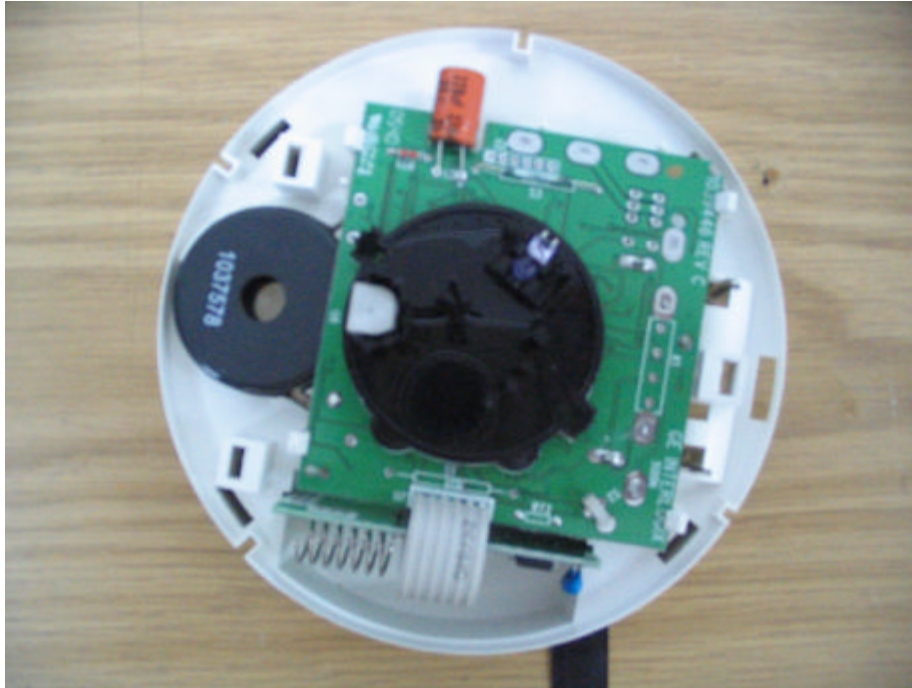
Photograph No.4 RWT30S433USA detector internal view without the second internal cover
