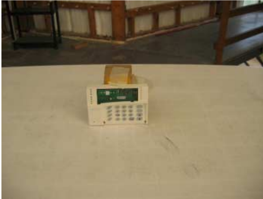
Photograph No.4 Spurious emissions field strength measurement setup, EUT view
