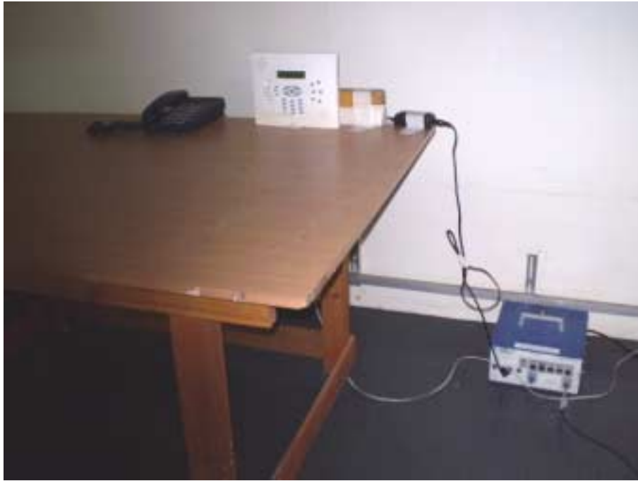
Photograph No.5 Setup for conducted emission measurements at the EUTpower port
