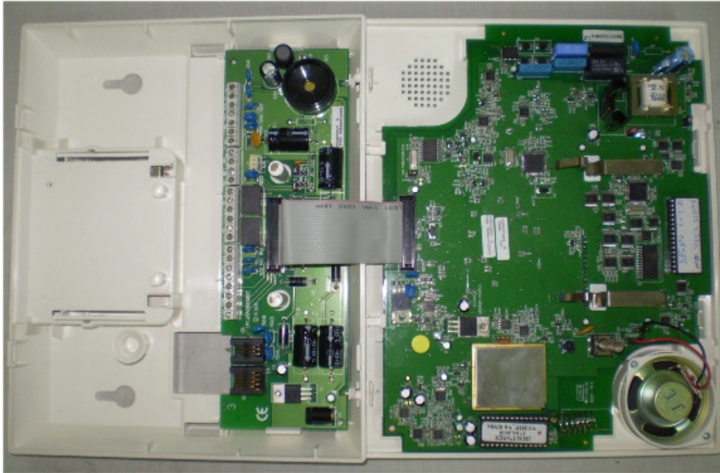
Photograph No.1 WisDom control panel internal view
