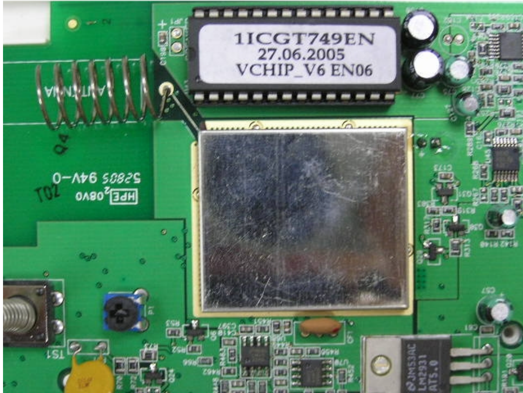
Photograph No.6 Antenna assembly
