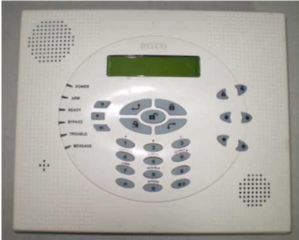
Photograph No.1 WisDom control panel front view
