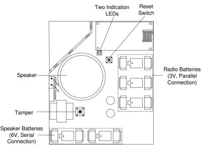
Internal Sounder - PCB Diagram
