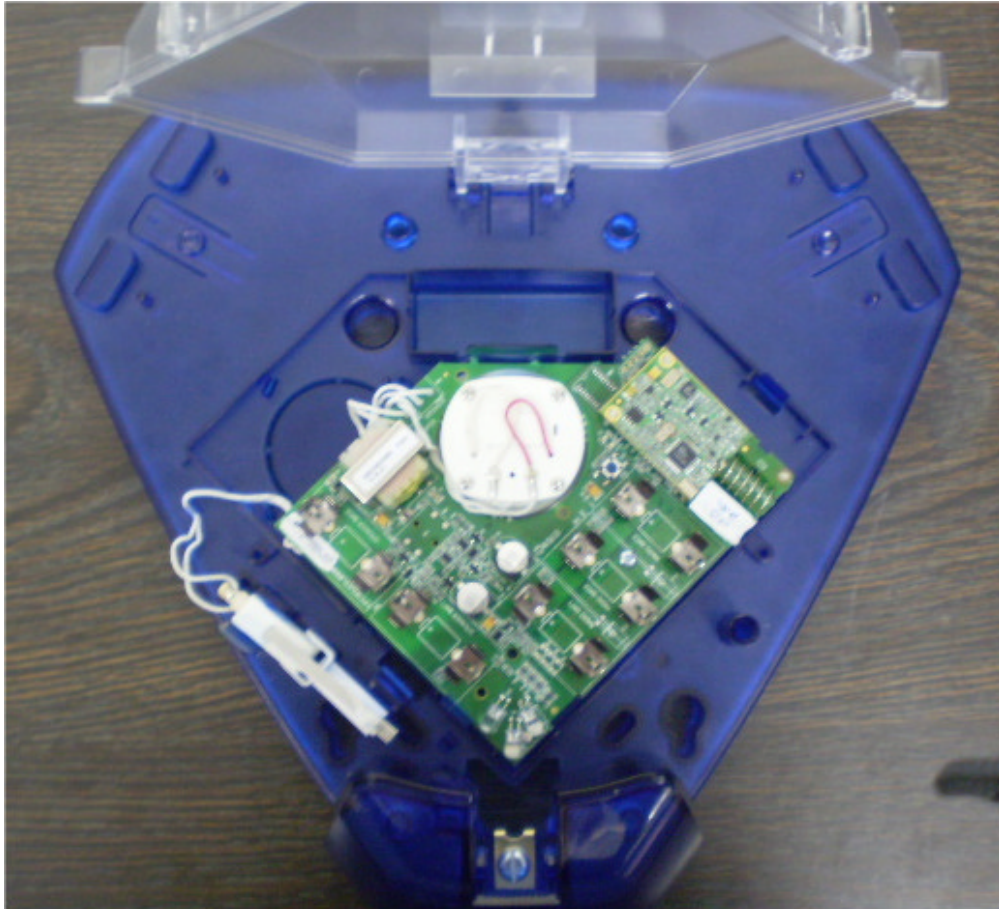
Photograph No.3 Siren internal view with cover removed
