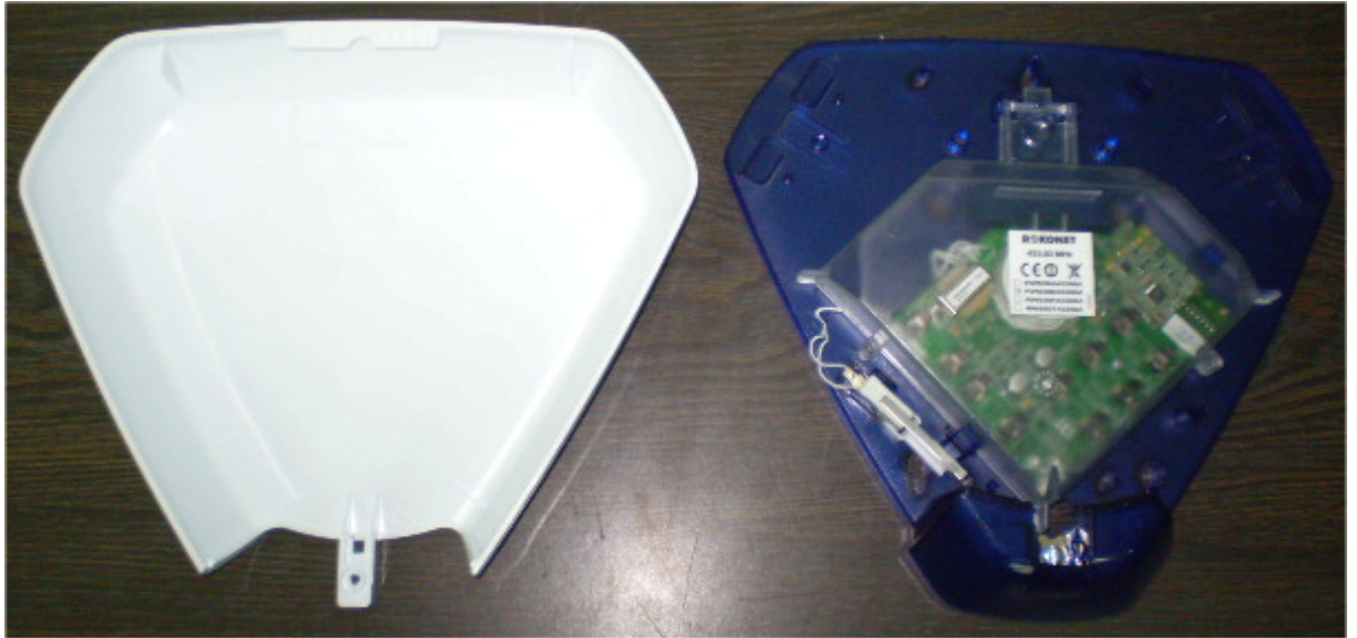
Photograph No.1 Siren internal view
