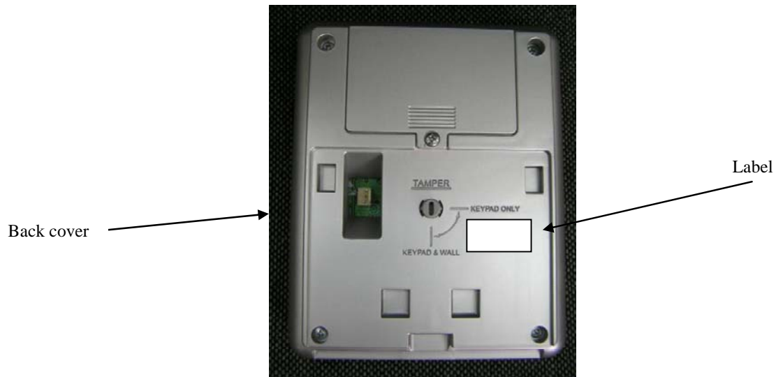
Figure 2. Location of Label on EUT
