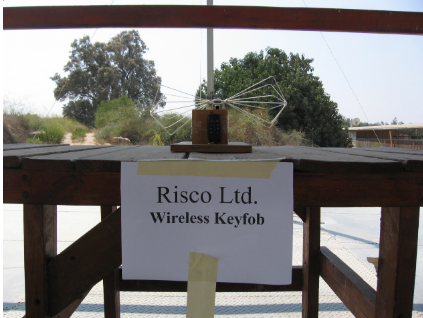
Figure 4. Radiated Emission Test
