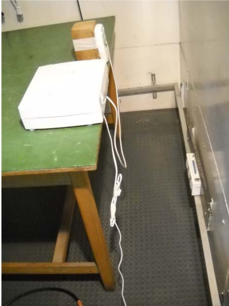
Photograph No.4 Setup for conducted emission measurements at the EUT power port
