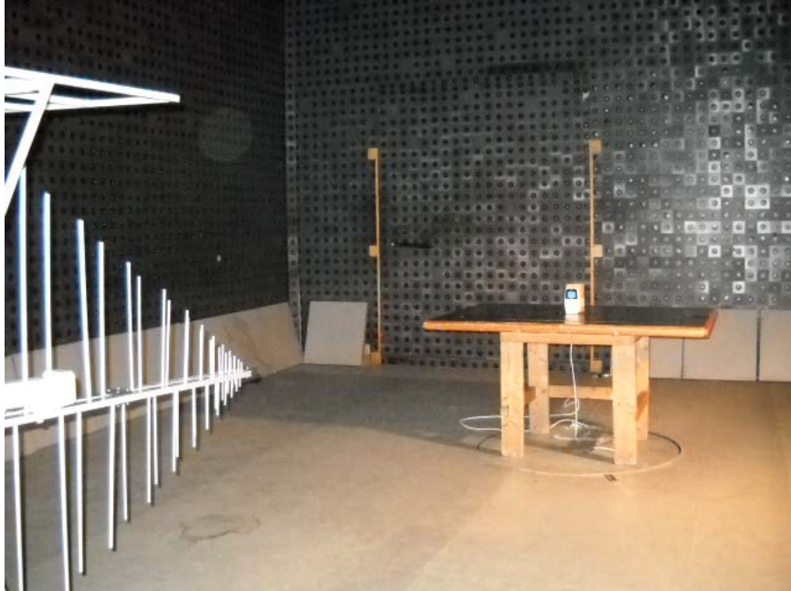
Photograph No.2 Spurious emission measurement test setup from 30 MHz to 1000 MHz in the anechoic chamber
