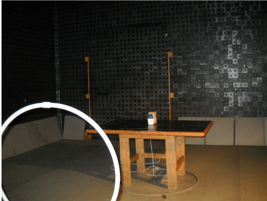
Photograph No.1 In-band emissions and spurious emissions field strength measurement setup below 30 MHz in the anechoic chamber
