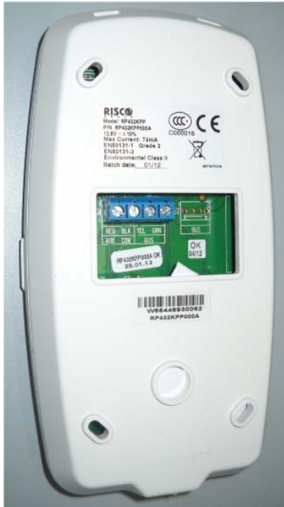
Photograph No.3 Keypad rear side view
