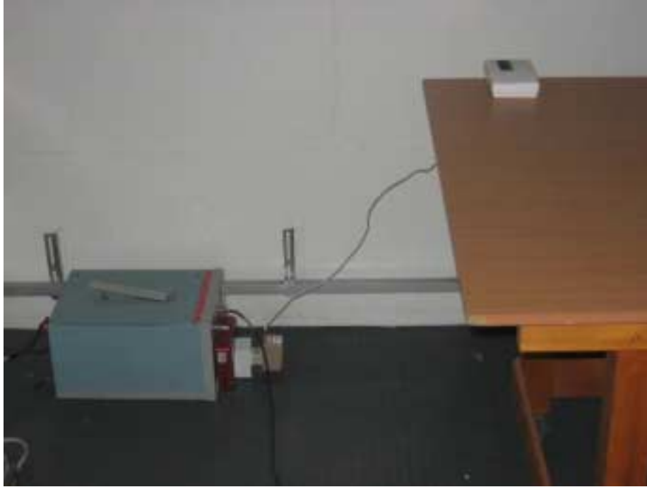
Photograph No.5 Conducted emissions measurement setup
