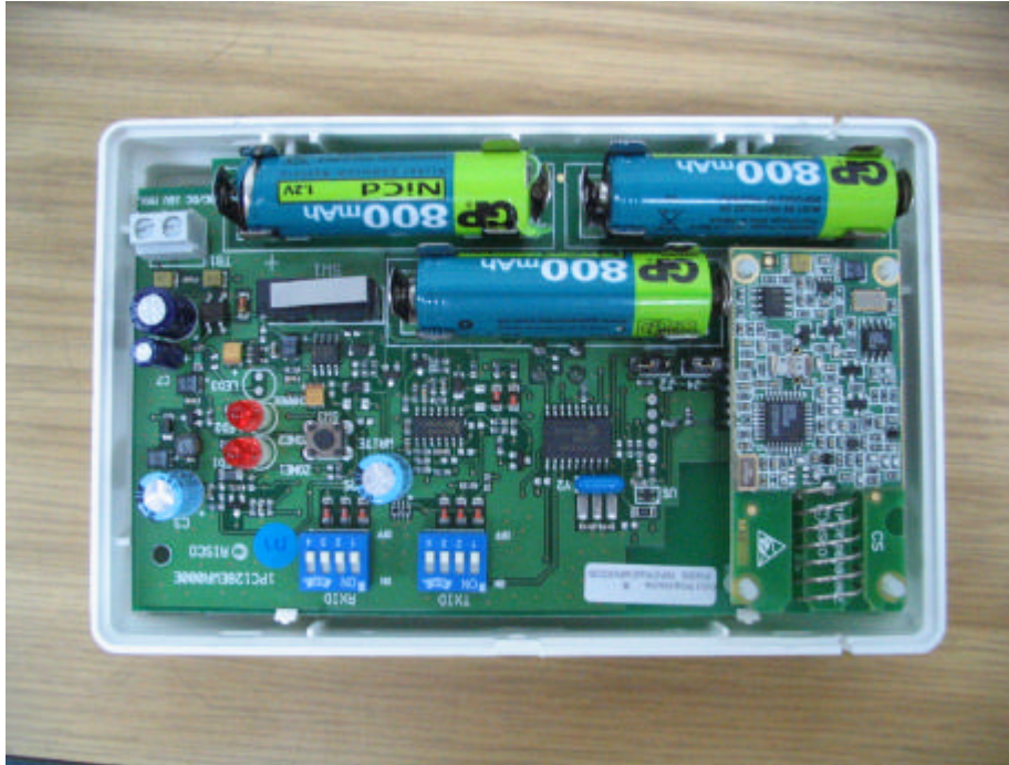
Photograph No.1 RP296EWR0USA repeater internal view
