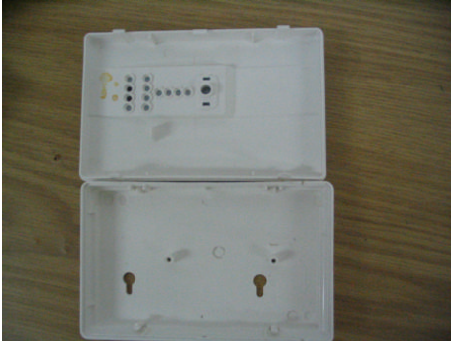
Photograph No.2 RP296EWR0USA repeater internal view of enclosure
