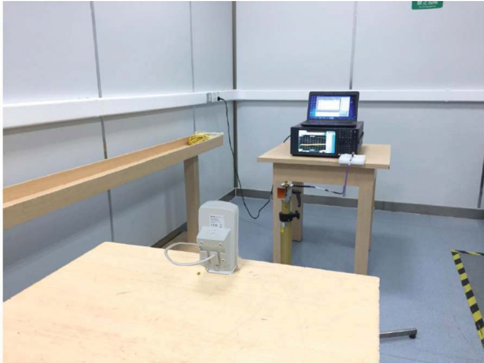
Description: Radiated Emission Test Setup for 40GHz ~ 60GHz
