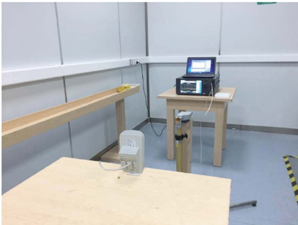
Description: Radiated Emission Test Setup for 60GHz ~ 90GHz
