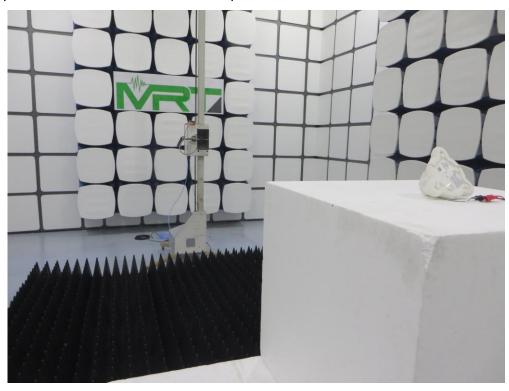
Description: Radiated Emission Test Setup for  $18G \sim 40GHz$
