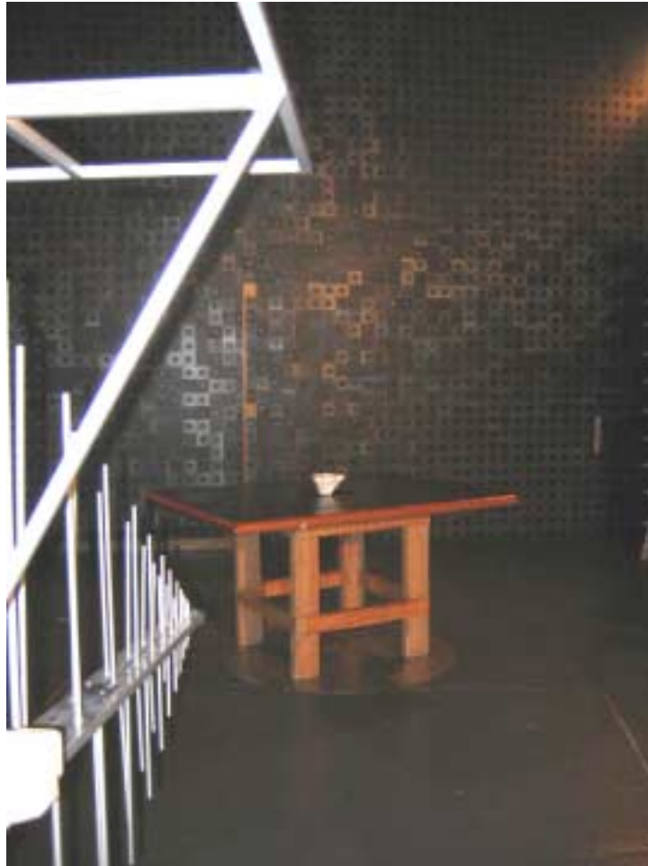
Photograph No.2 Radiated emission measurement test setup from 30 to 1000 MHz
