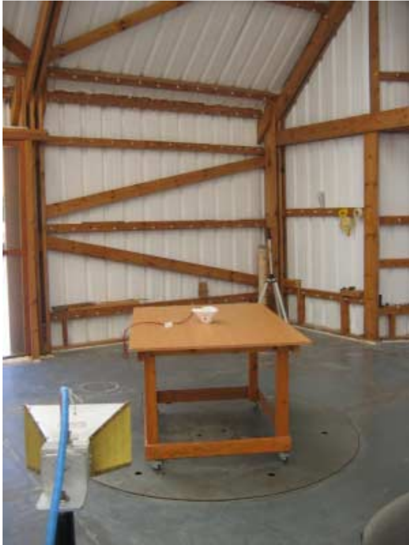
Photograph No.6 Band edge emission measurement setup
