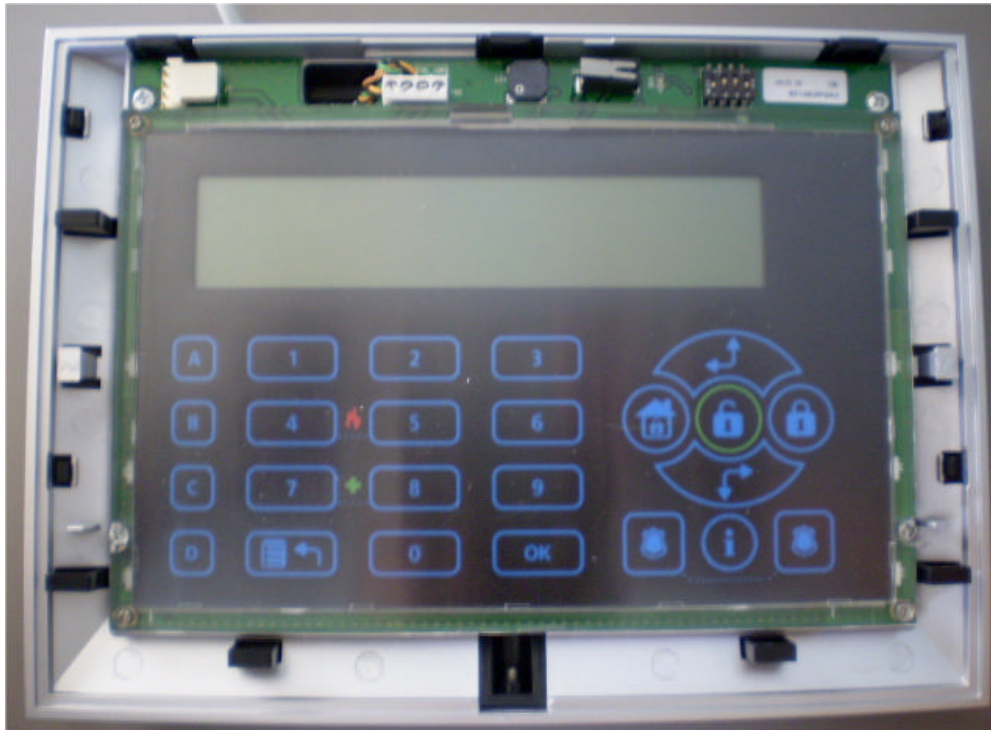
Photograph No.1 Touch screen keypad internal view
