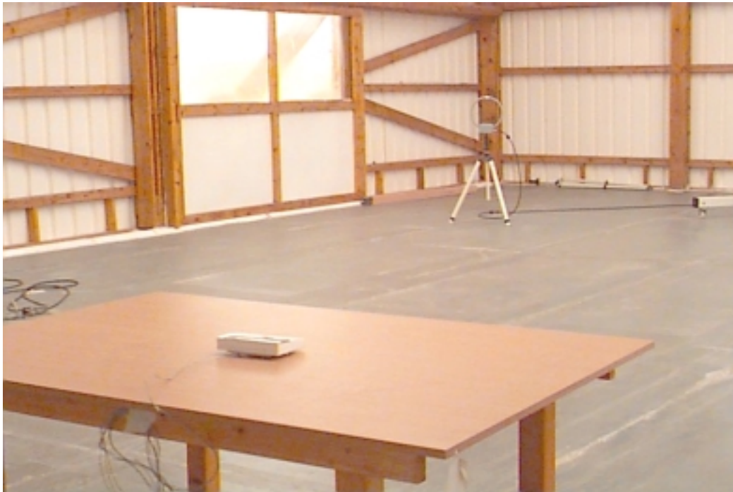
Photograph No.1 Radiated emissions measurement test setup
