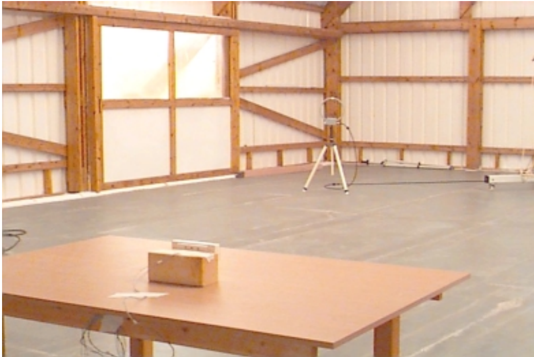
Photograph No.3 Radiated emission measurement test setup
