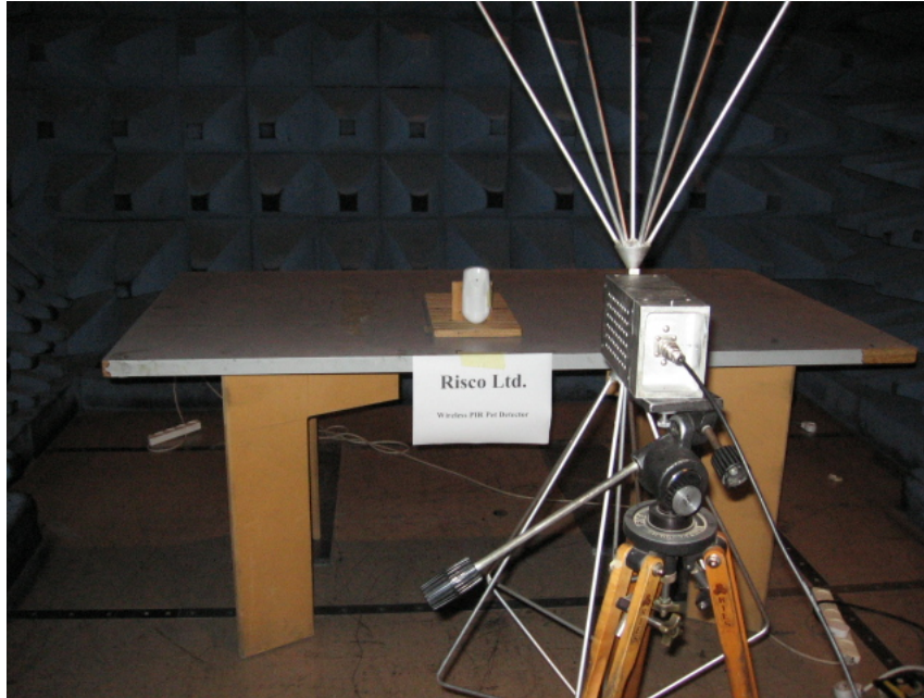
Figure 2. Radiated Emission Screening Test, Host: Two Way Wireless PIR Detector
