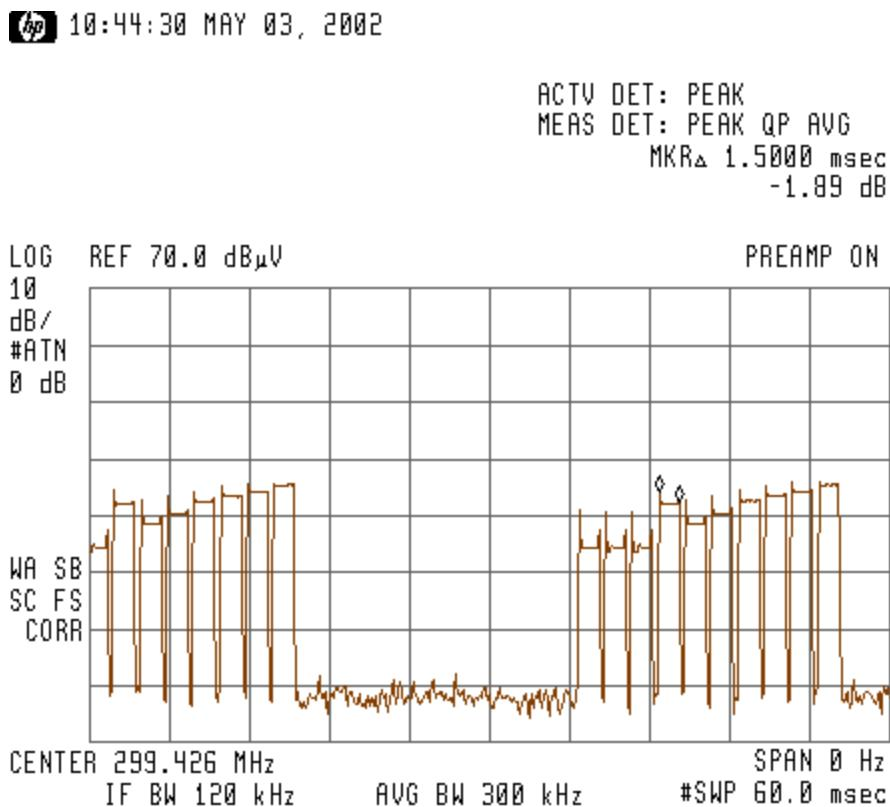
Given 10 wide peaks of 1.5ms, and a transmission length of 40.8ms, we can perform the average factor calculation.
