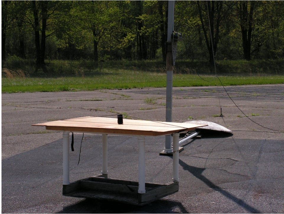
Photograph 6.5. DUT on OATS (one of three axes tested, one of three models tested)
