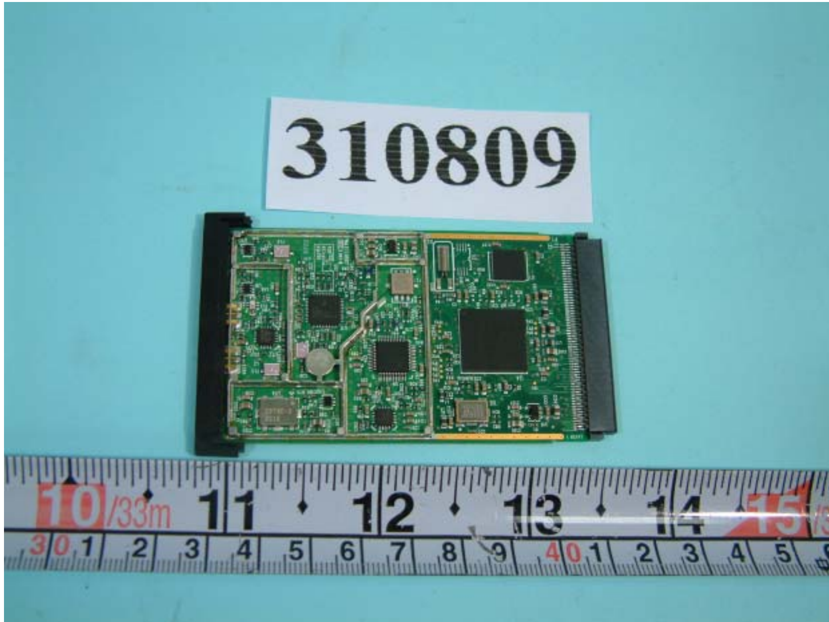
Front side of Main Board of RF Module
