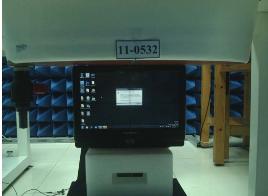
Figure 3. Body SAR Test Setup (Edge Top to phantom)
