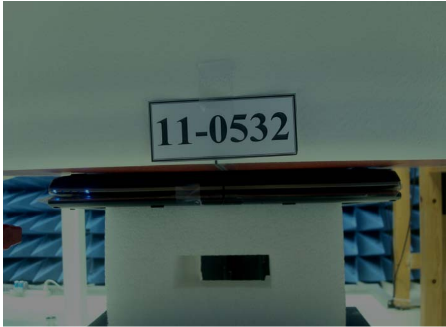
Figure 1. Body SAR Test Setup (Back Surface to phantom)
