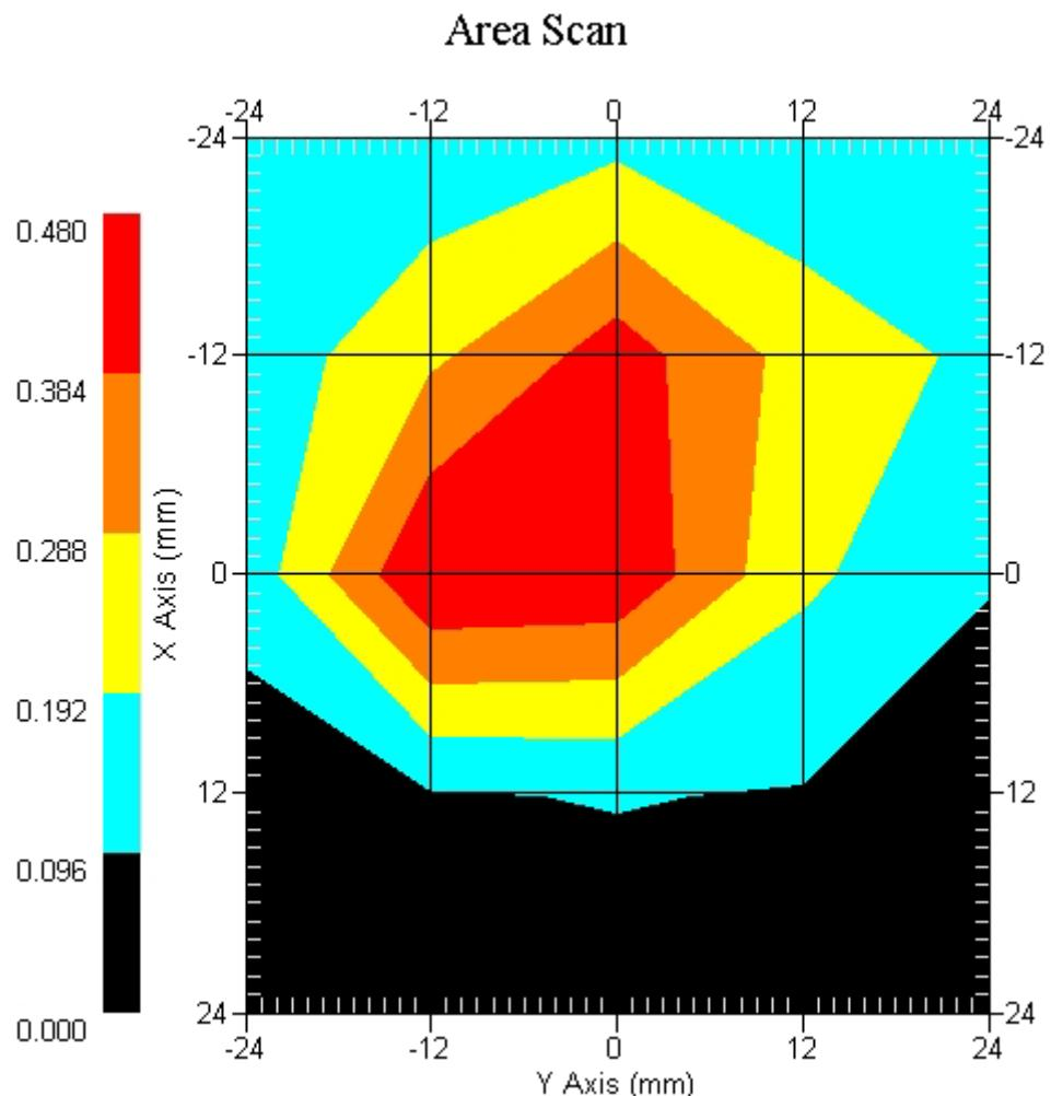
**802.11b-Tx2 Antenna, EUT Top Z-Axis plot****Channel: 6**
