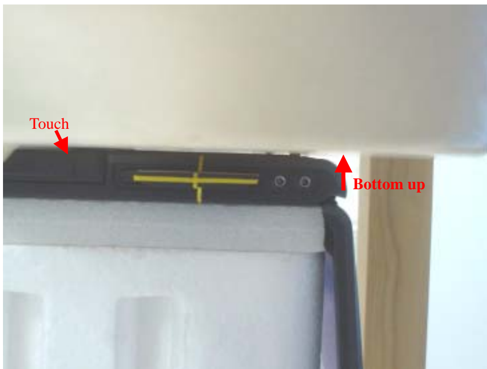
Fig.4 Photograph of the Bottom face of the notebook is paralleled with flat phantom. Spacing between EUT and phantom - In contact (10 mm)
