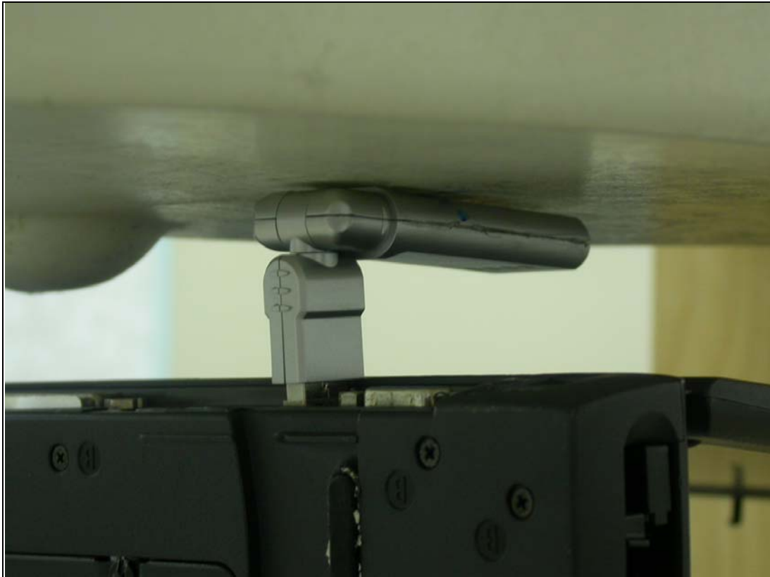
The front side of the EUT to the flat phantom distance 0mm
