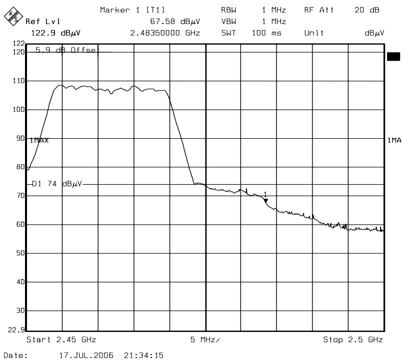
**Detector mode: Average    Polarity: Horizontal**
