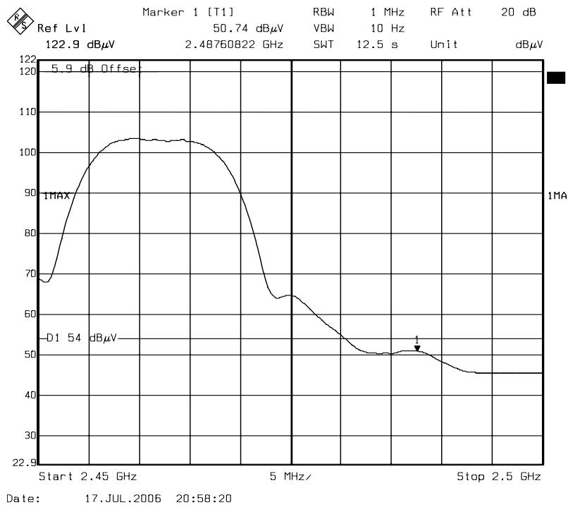
**Band Edges (IEEE 802.11g mode / CH Low)****Detector mode: Peak    Polarity: Vertical**
