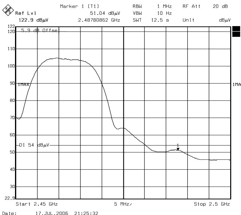
**Detector mode: Peak    Polarity: Horizontal**
