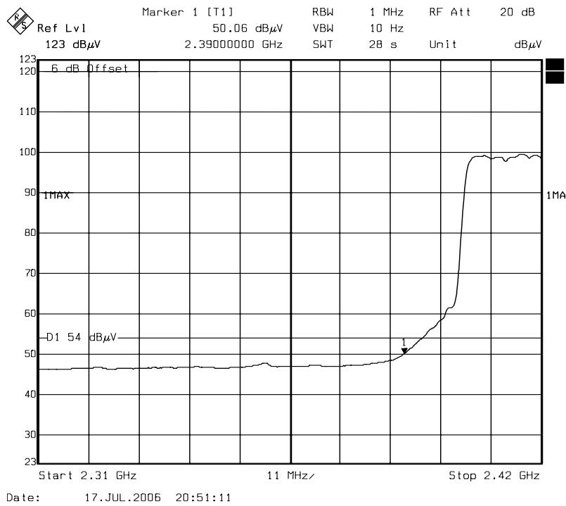
**Band Edges (IEEE 802.11g mode / CH High)****Detector mode: Peak    Polarity: Vertical**
