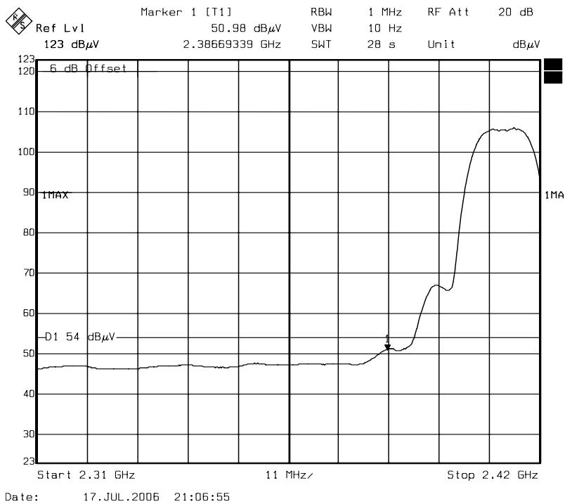
**Band Edges (IEEE 802.11b mode / CH High)****Detector mode: Peak    Polarity: Vertical**
