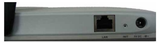
The Access Point's ports are located on the Access Point's rear panel.
