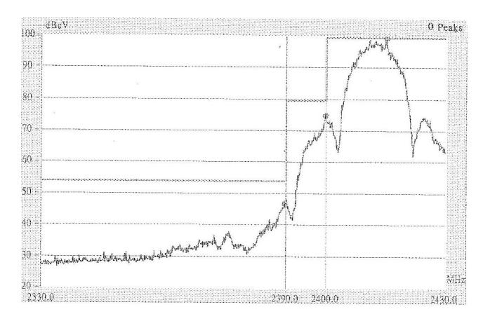
This is the hard copy of our bandedge measurement generated by our bandedge testing program. The picture shown above is the bandedge of channel 1.
