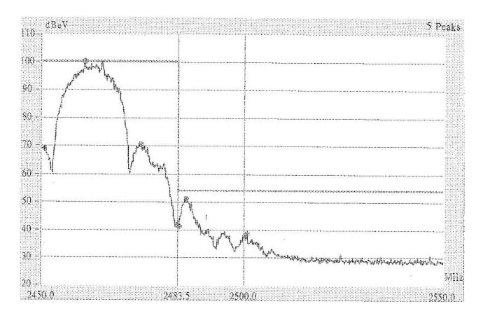
This is the hard copy of our bandedge measurement generated by our bandedge testing program. The picture shown above is the bandedge of channel 11.
