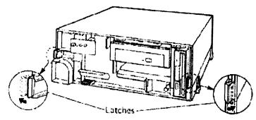
4 With the latches pressed outwards, push the cover towards the real panel and remove it.
