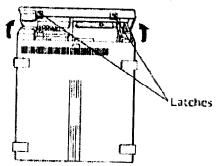
Press the latches on the sides of the personal computer outwards.
