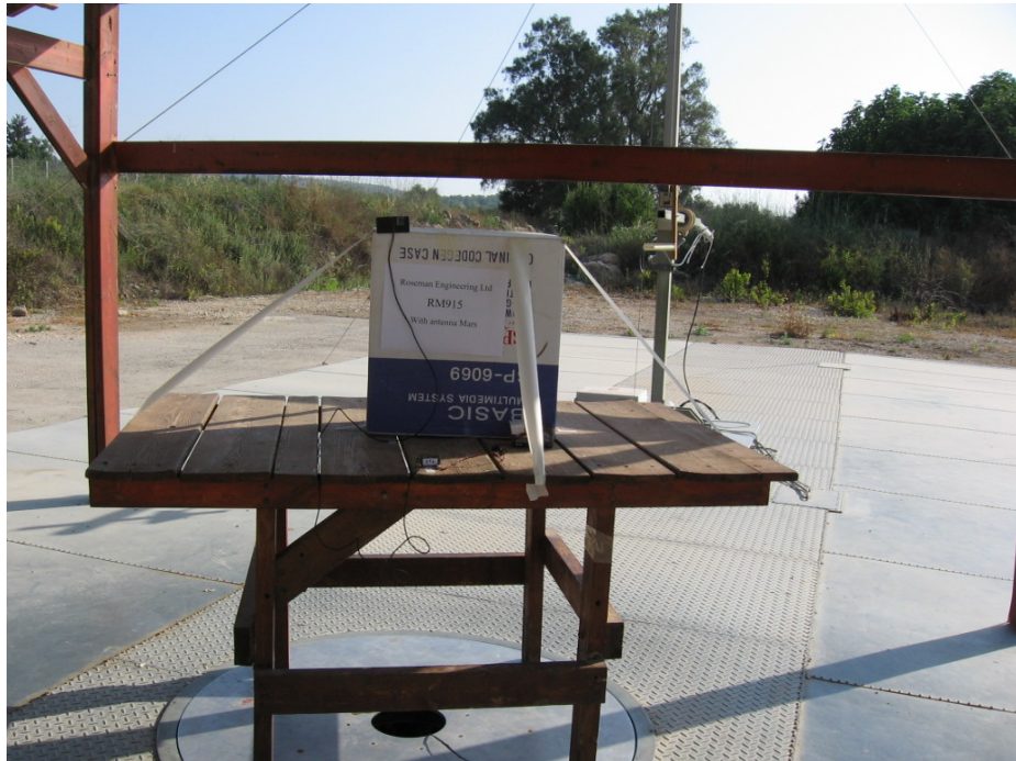
Figure 3. Radiated Emission Test Mars antenna
