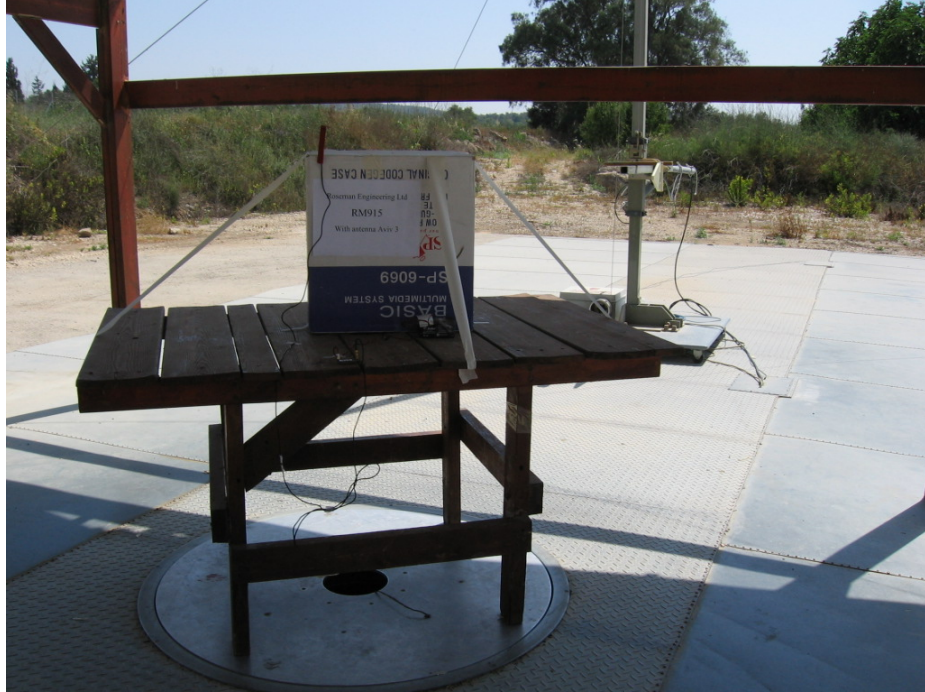
Figure 2. Radiated Emission Test Aviv 3 Antenna
