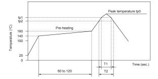
Measuring point of temperature : IN-OUT Terminals of The Device Reflow Soldering : Both Convection and Infrared Rays, Hot Air and Hot Plate
