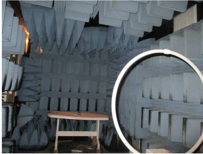
Figure 1. Radiated Emission Test, 0.009-30.0 MHz
