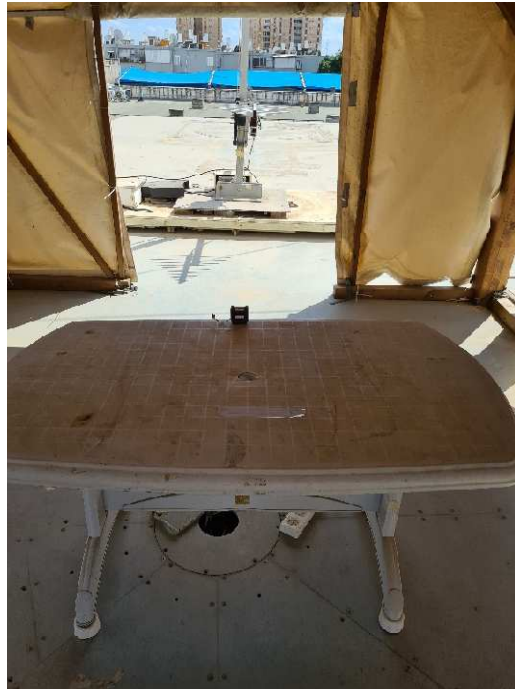
Figure 3. Radiated Emission Test, 200.0-1000.0 MHz
