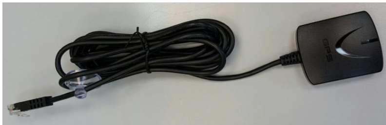
Figure 11 GPS Antenna Cable
