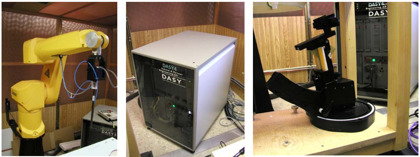
Figure 5-1 DASY4 system: Robot Arm, Controller box, Device Positioning Holder
