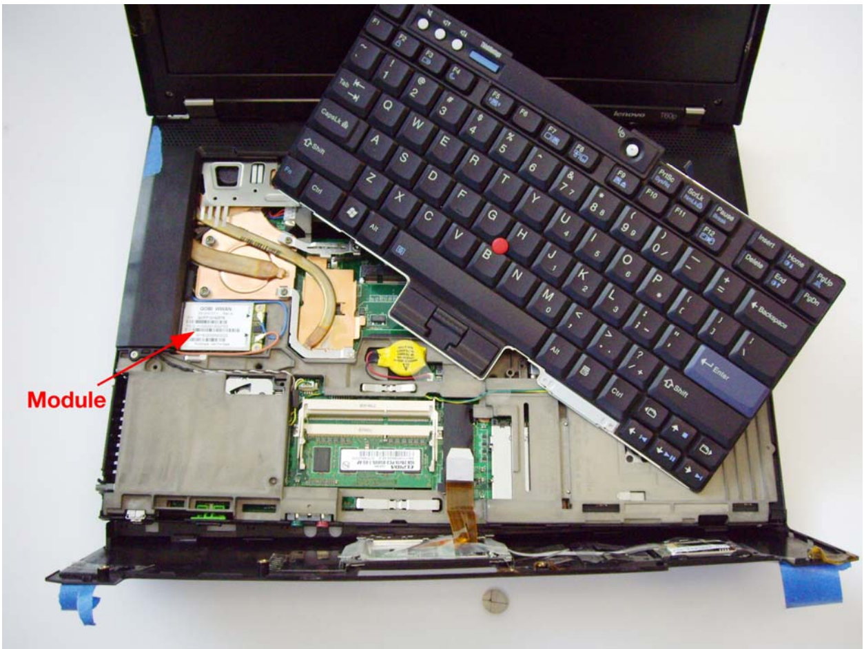
Figure 12-3 Internal View of Notebook with Module Exposed
