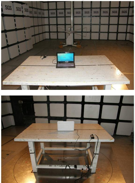
**Radiated Emission Set up Photos**
