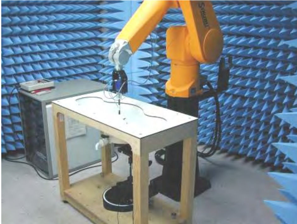
Fig.1 Photograph of the SAR measurement System
