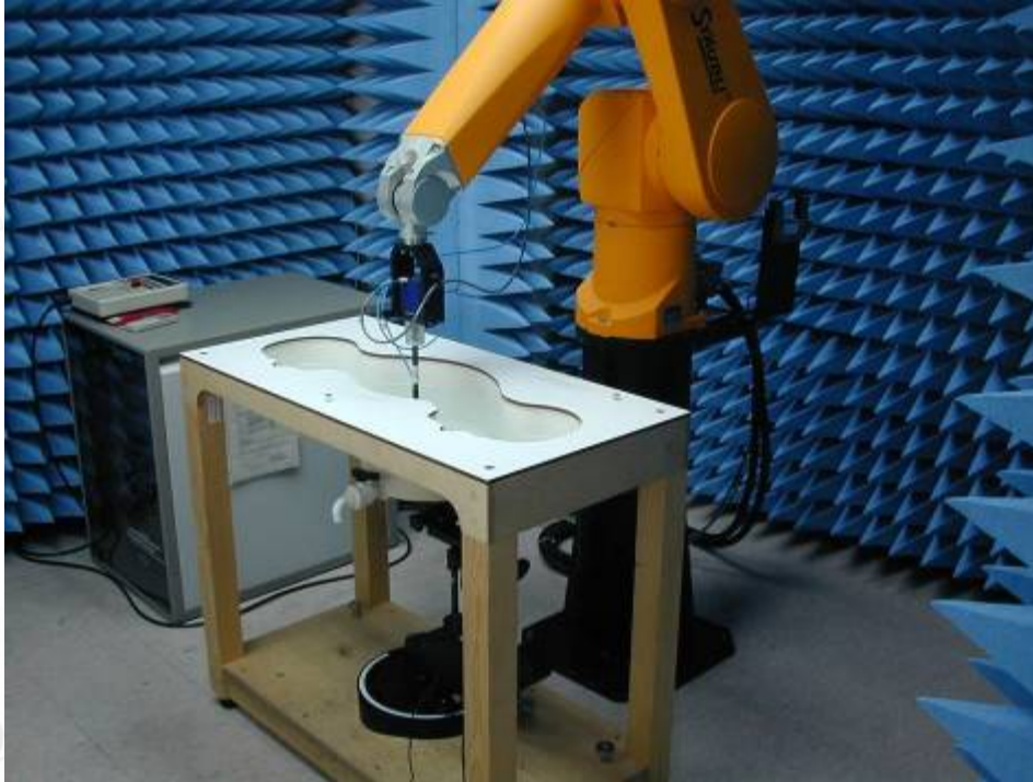
Fig.1 Photograph of the SAR measurement System
