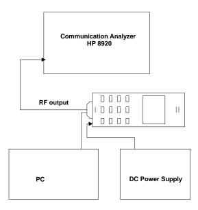
**Definition** - The output power rating of the transmitter is the power available at the output terminal of the transmitter when the terminal is connected to the normal load.
