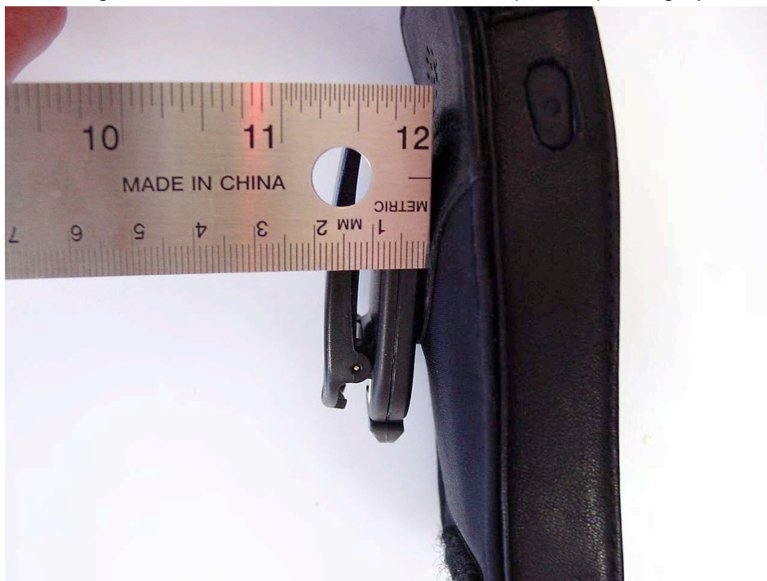
Figure A-8 Side view of leather holster 700-47205-0002 (not tested) showing clip dimension
