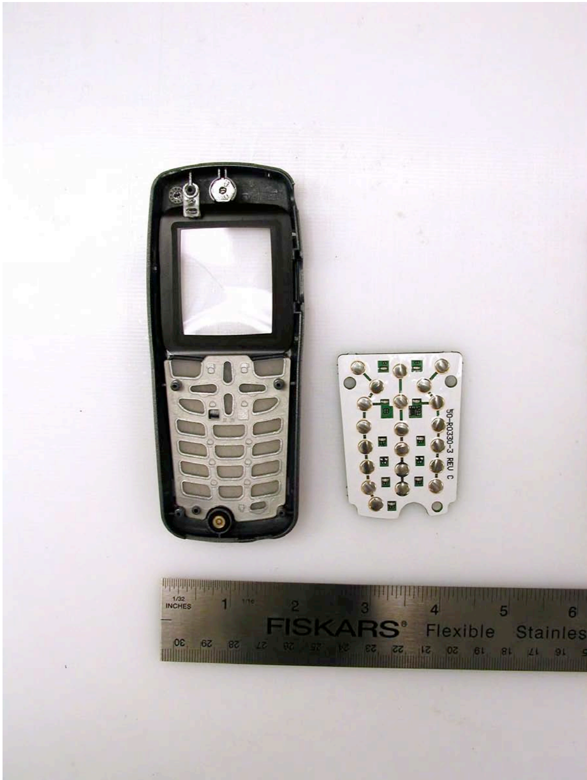
Figure 2-10 Front housing with keypad printed wiring board removed
