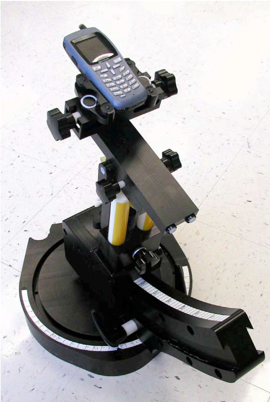
Figure 6-1 Phone in positioning device (view 1)
