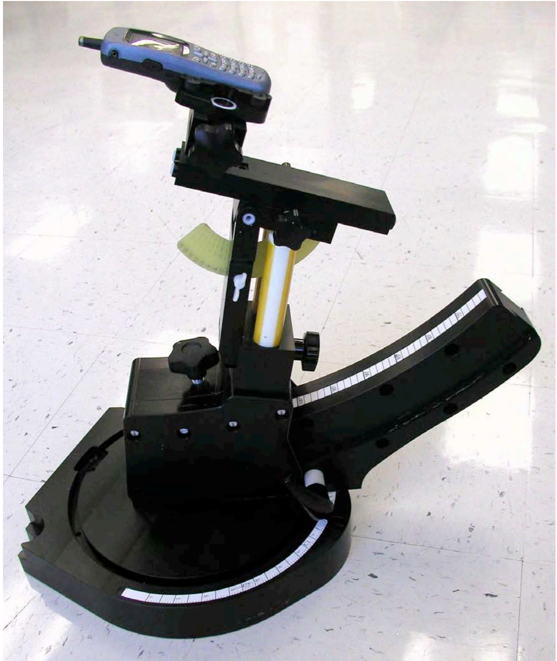
Figure 6-2 Phone in positioning device (view 2)
