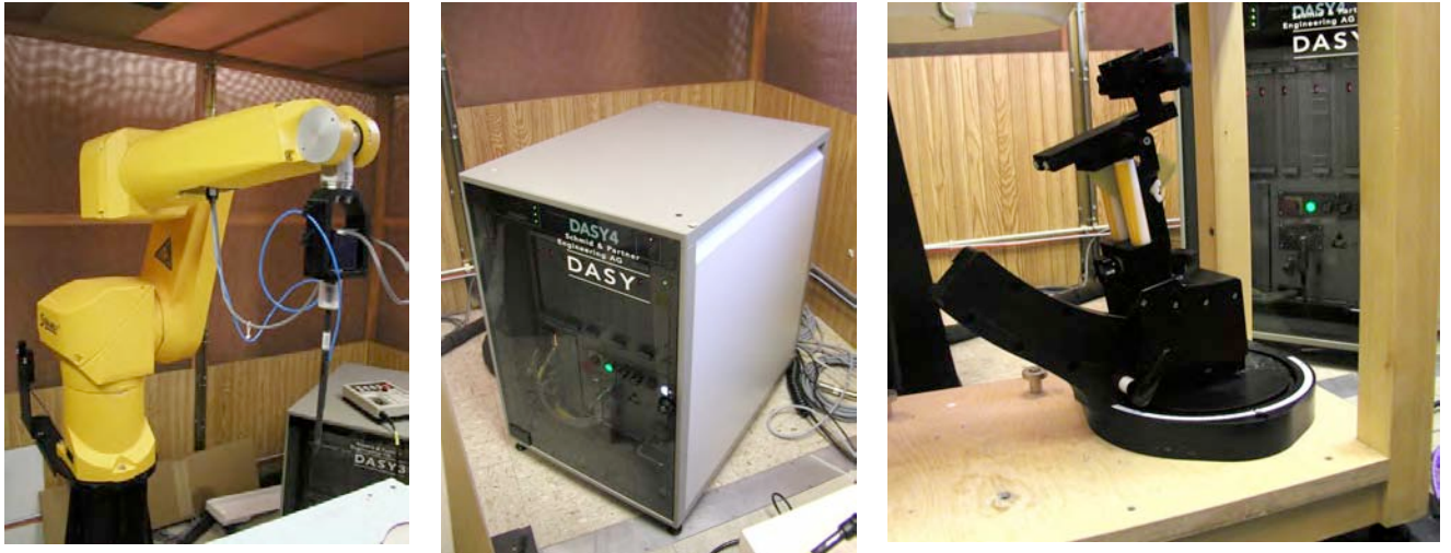
Figure 3-1 DASY4 system: Robot Arm, Controller box, Device Positioning Holder
