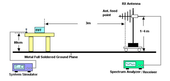
For radiated test above 1GHz
